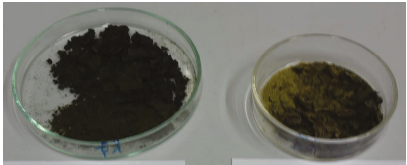
Figure 6. Dried biomasses from cultivation of Synechocystis sp. IFA-3 (left) and Chlorogloeopsis sp. Heinrichs-4 (right) in the 5-L tubular photobioreactor.
