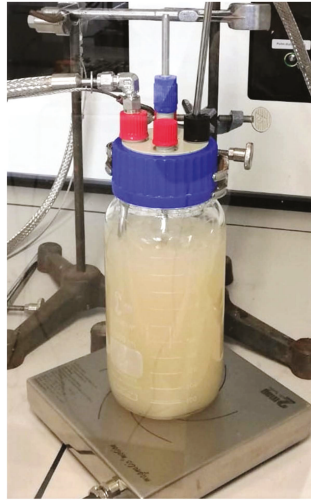
Figure 2. Explosion-proof bioreactor setup consisting of a 1 L DURAN® bottle with a magnetic anchor stirrer on a magnetic stirrer plate. Gas substrate is supplied by a steel tube with a PTFE frit at the end.
