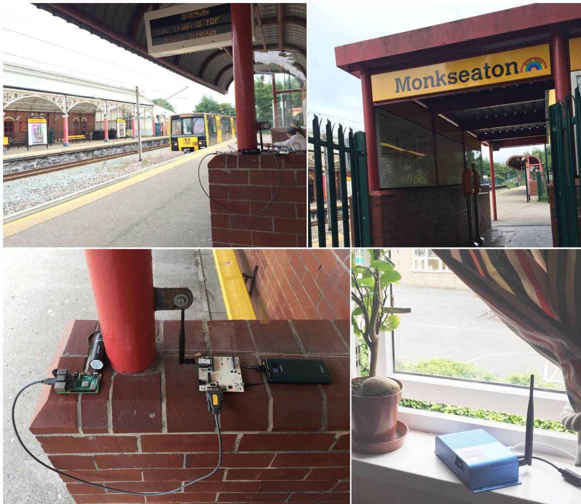
Fig. 5.2 The Monkseaton Metro station with the experimental TrainBusters hardware setup at the platform; a LoRa base station on a kitchen's window sill.
