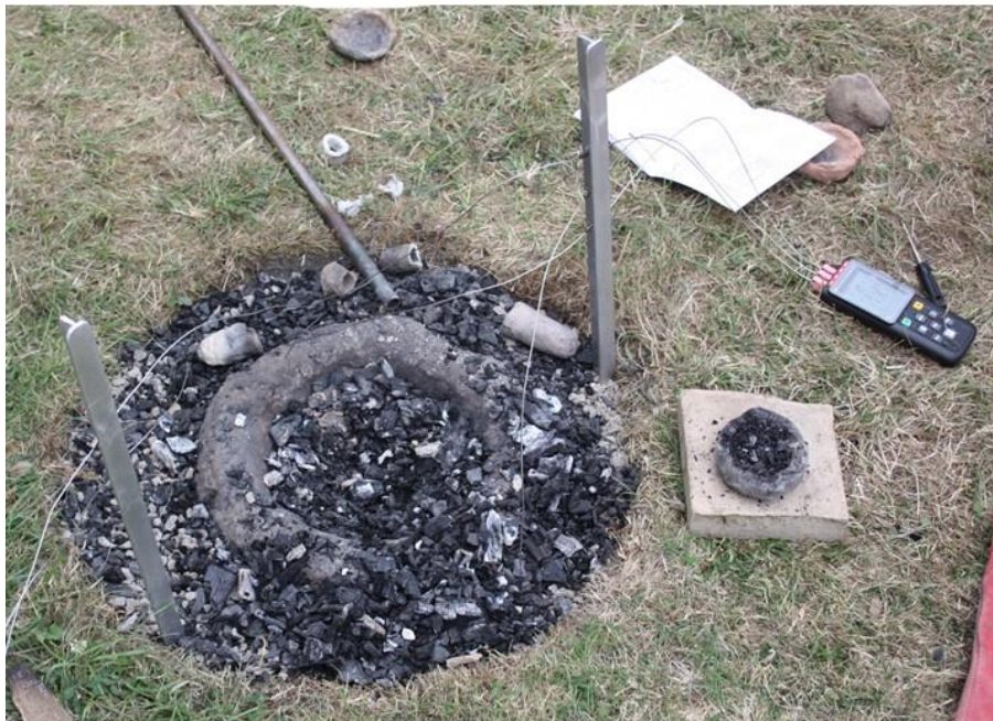
Figure 6.6 Thermocouples set-up used during JH-SMLT III-IV.
