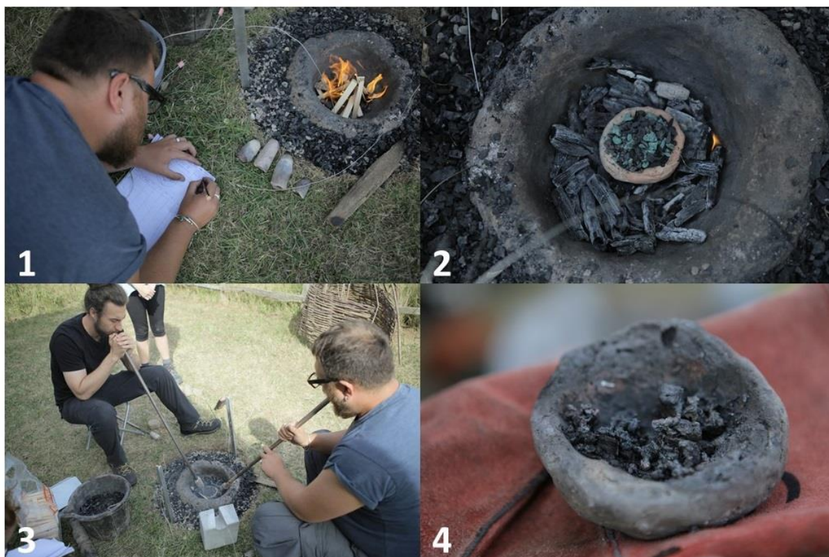
Figure 6.7 JH-SMLT IV: 1) experimental diary; 2) mixed bornite/malachite charge; 3) two blowpipe-operators; 4) crucible content at the end of the experiment.
