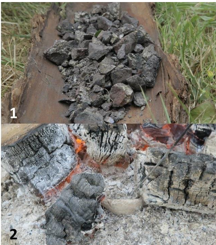
Figure 6.3 JH-RST II: 1) crushed ore; 2) crucible containing the most minute particles.
