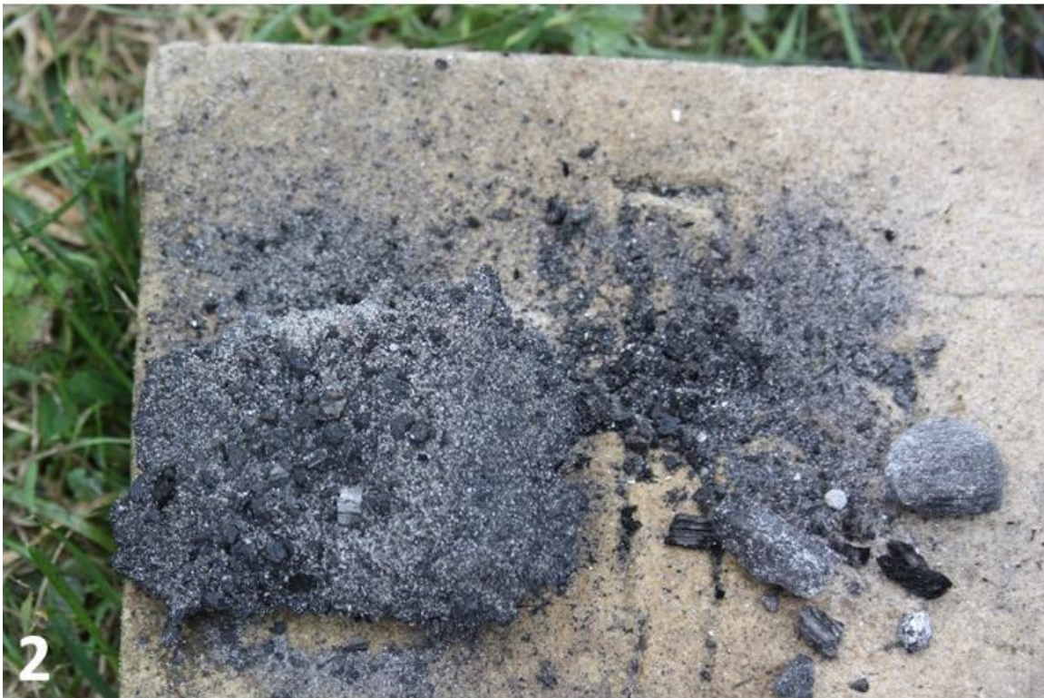
Figure 6.8 JH-SMLT VI: 1) crucible recovered from the furnace; 2) content of the crucible consisting of loose grain of unreacted ore and sand.
