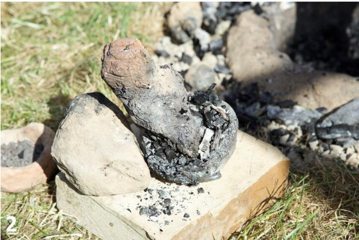
Figure 6.5 JH-SMLT I: 1) vitrified nozzles; 2) nozzle melted with crucible.
