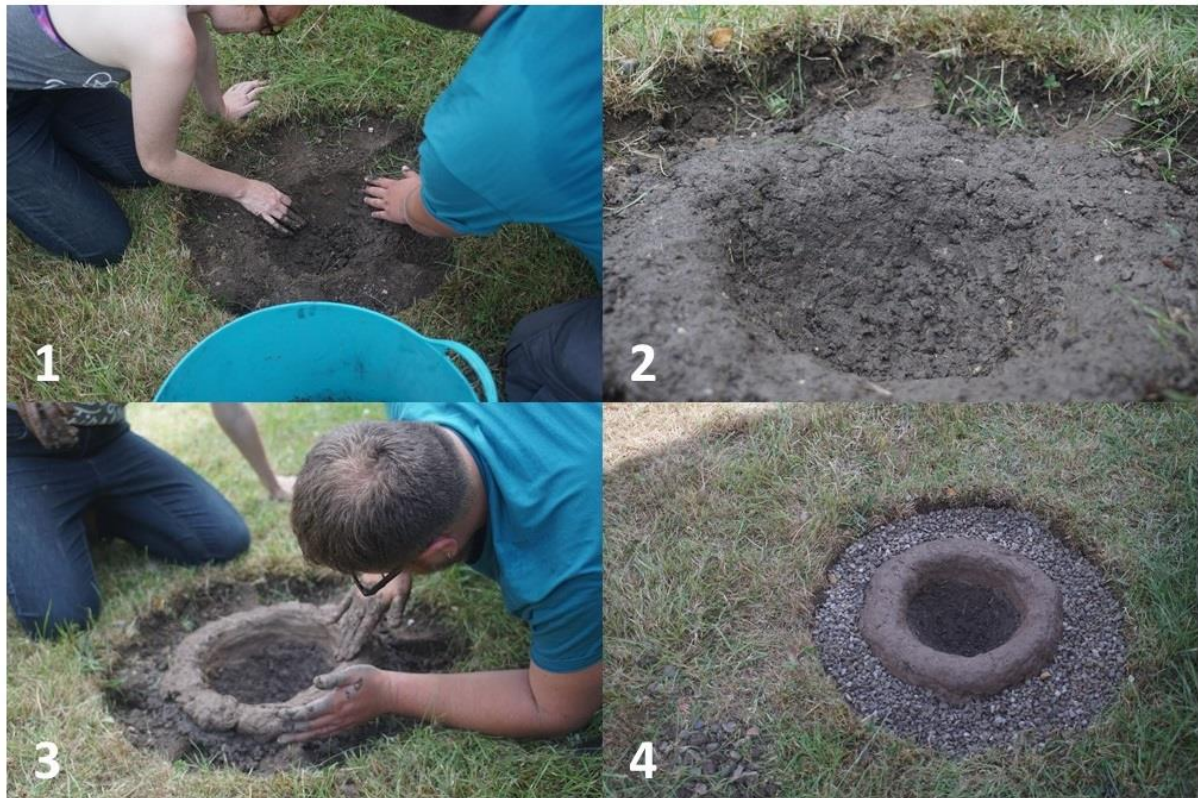
Figure 6.1 Bowl-shaped furnace's construction sequence.
