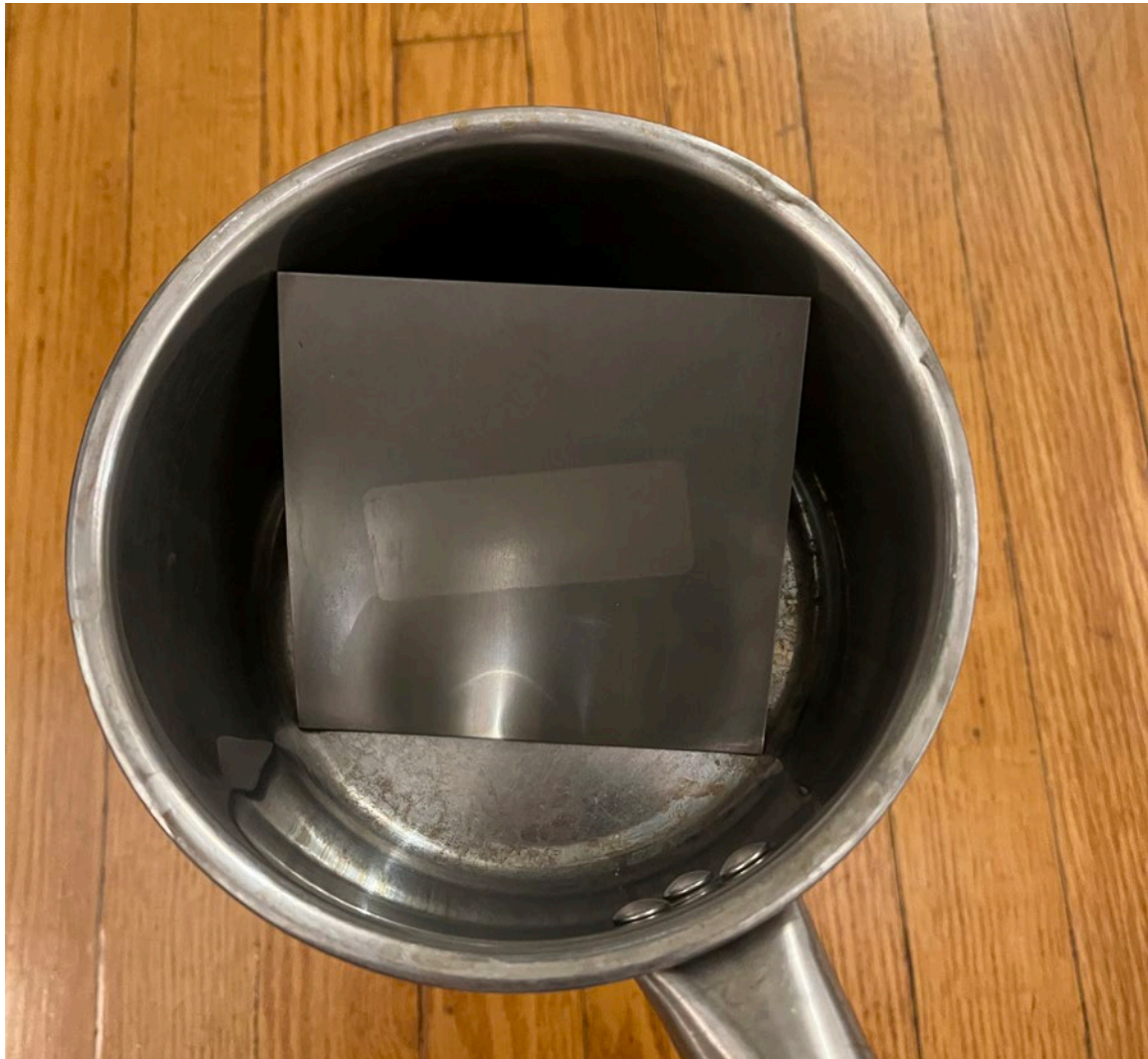
Base Material : Weathering steel, smooth Applied Material : N/A Accelerator : Salt water (direct) Temperature : Boiling point Time : 15 minutes
