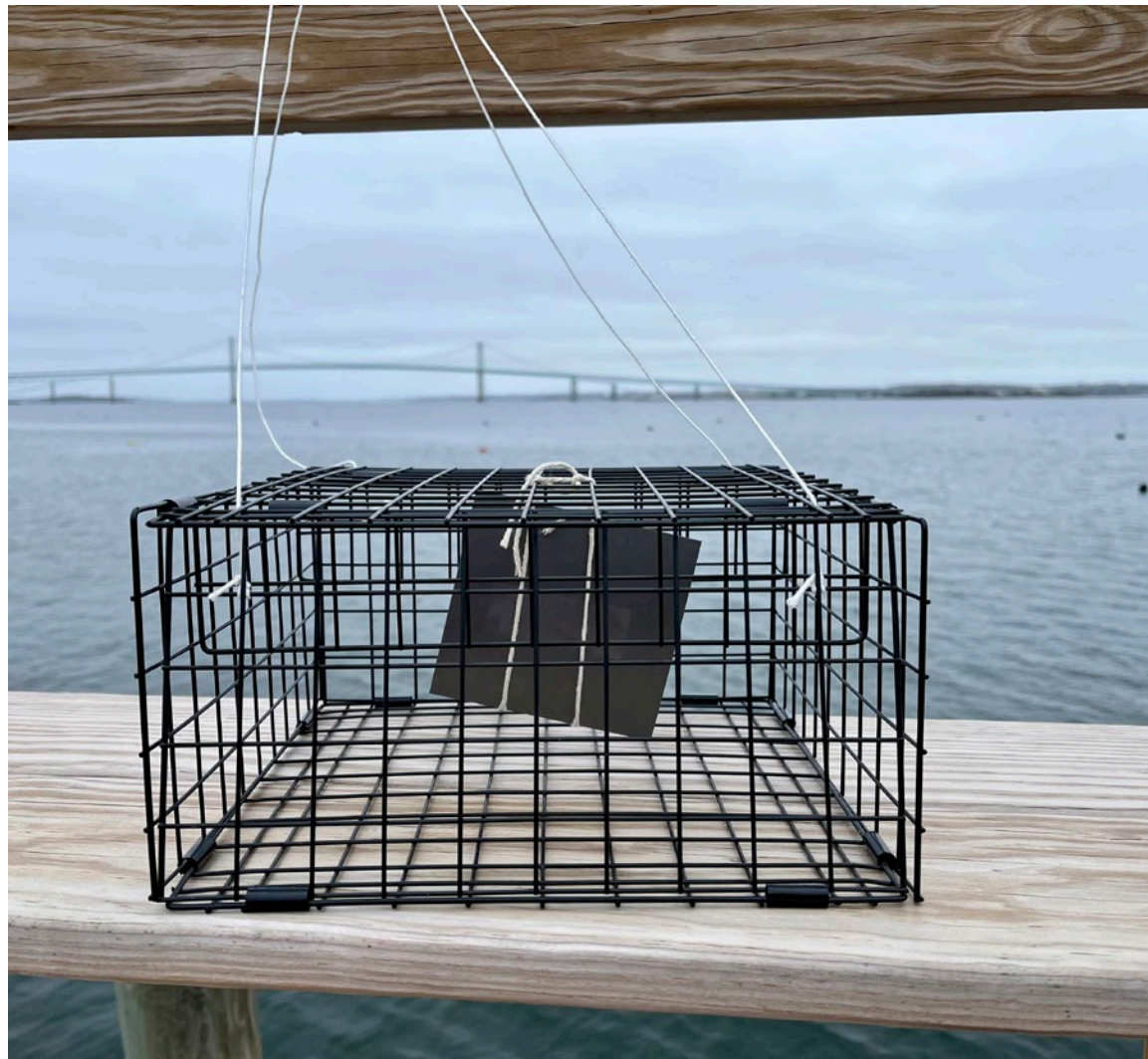
Base Material : Weathering steel, smooth Applied Material : N/A Accelerator : Narragansett Bay Water Temperature : ~48 degrees Time : 1 hour, but continued to rust after
