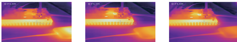
Fig. 28. Heat sink thermal image of the converter with the Si IGBT at 800 V of v_{in} and switching frequency of 20 kHz (left), 50 kHz (middle), and 100 kHz (right).
