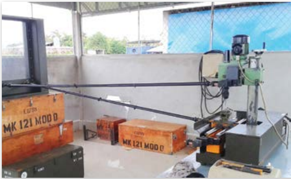
Figure 4. Mechanical Remote Fuze Disassembly Kit used for removing small energetic components such as primers in fuze rotors, GWHF Cambodia 2014. If mine action organizations wish to make items of explosive ordnance INERT, and to train suitable staff to do so, specialist explosive processing facilities are required.
