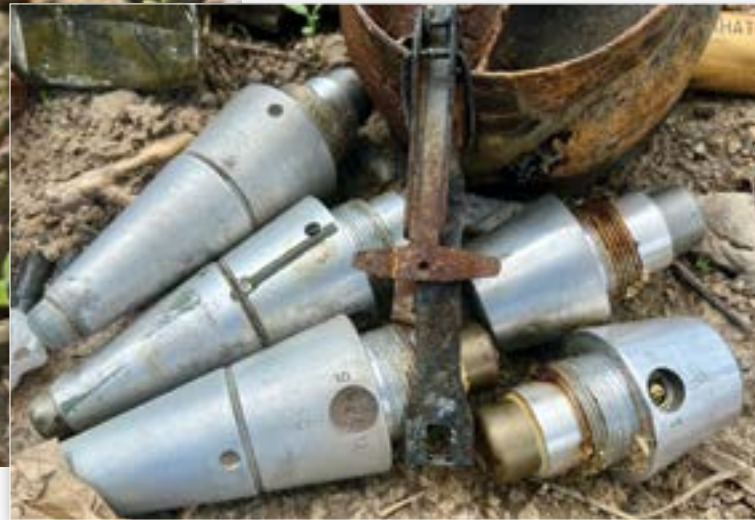
MRV-U impact fuzes for grad system. Image courtesy of HALO.
