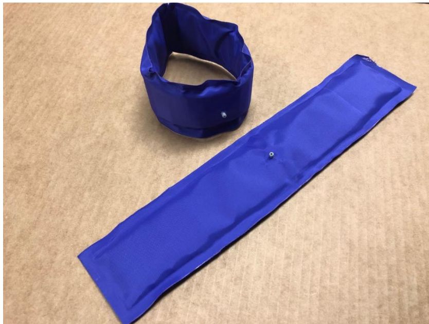
Figure 31: Air bladders with straw internal structure.
