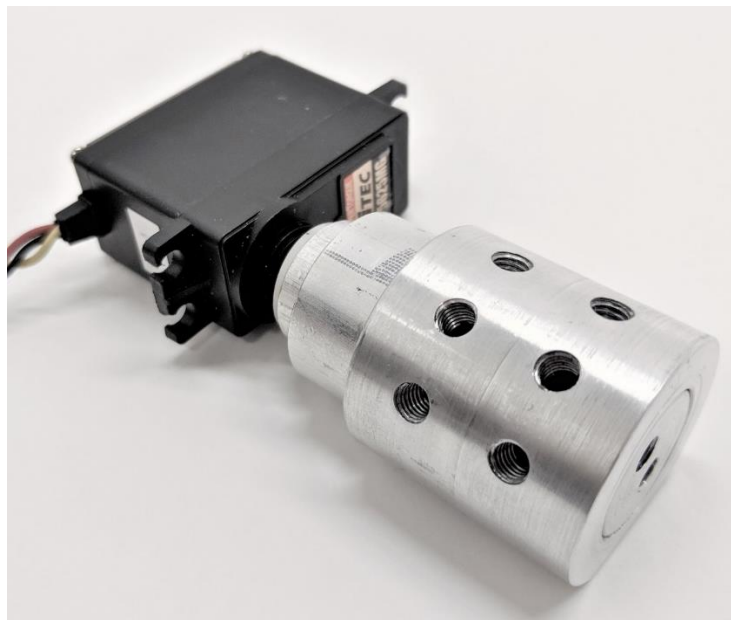
Figure 10: Final rotating valve iteration with attached Servo motor.
