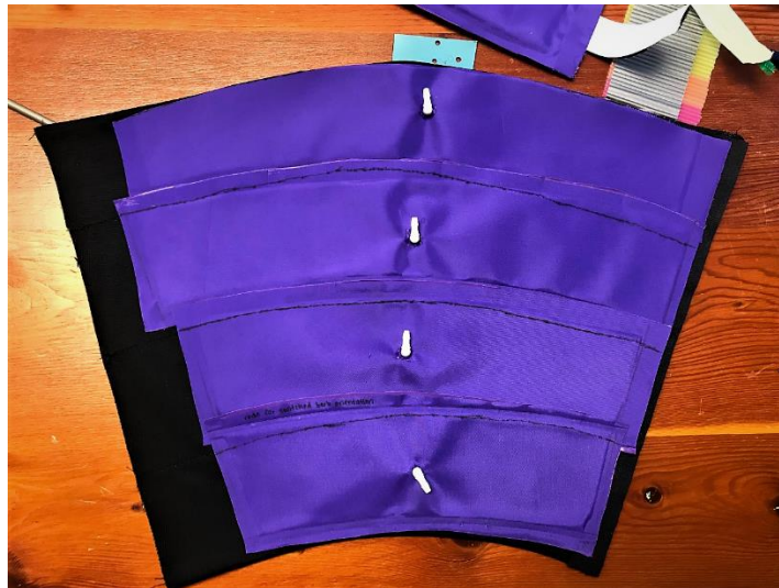
Figure 8: Curved airbags with tube fittings.
