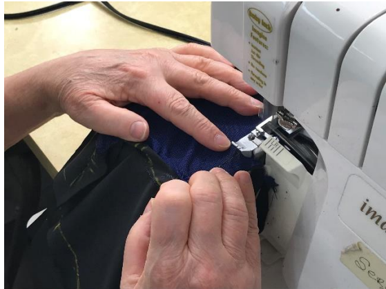
Figure 22: Sue Bonde attaching the non-compressive stretch mesh to the garment using a serger.
