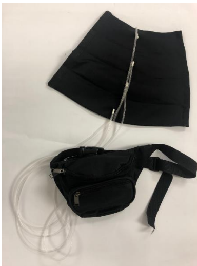
Figure 16: Final iteration of outer airbag wrap with channeled pockets, alongside fanny pack containing electrical and mechanical components.
