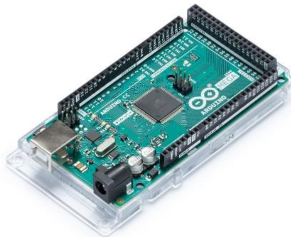
Figure 11: Arduino Mega 2560 with 54 digital I/O pins for wide range of control capabilities and combinations [15].
