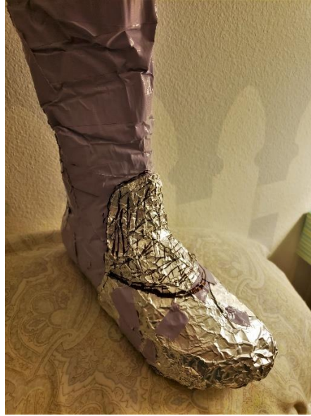
Figure 19: Aluminum foil layering onto last for patterns.
