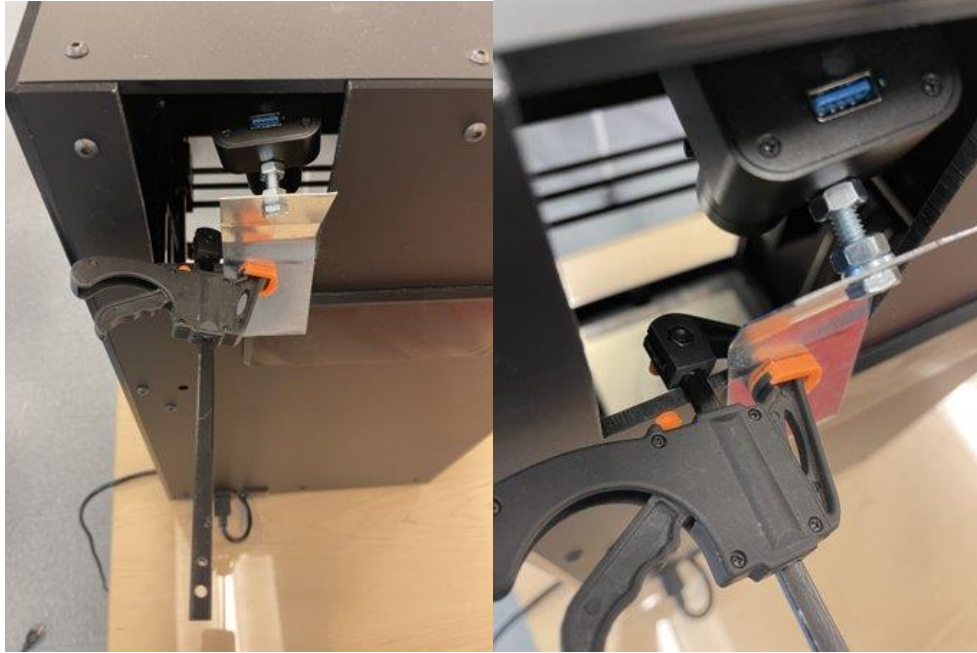
Figure 3: Camera mounted in the back panel sent from Hydra Research, LLC. We moved to a small piece of sheet metal that holds the camera at a more consistent angle than the previous gooseneck design. As can be seen in this image, there is still plenty of room for the USB connection to the camera, and the metal can be bent backwards or forwards for slight adjustments.
