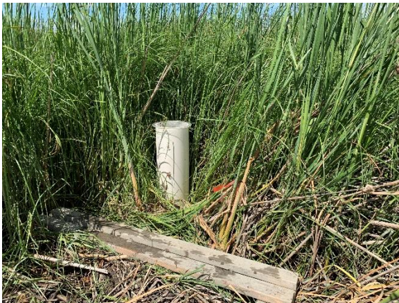
Figure 36. Static chamber in tall vegetation with bench set-up (a) Static chamber gas sample collection through septum (b)
