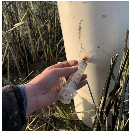
Figure 36. Static chamber in tall vegetation with bench set-up (a) Static chamber gas sample collection through septum (b)
