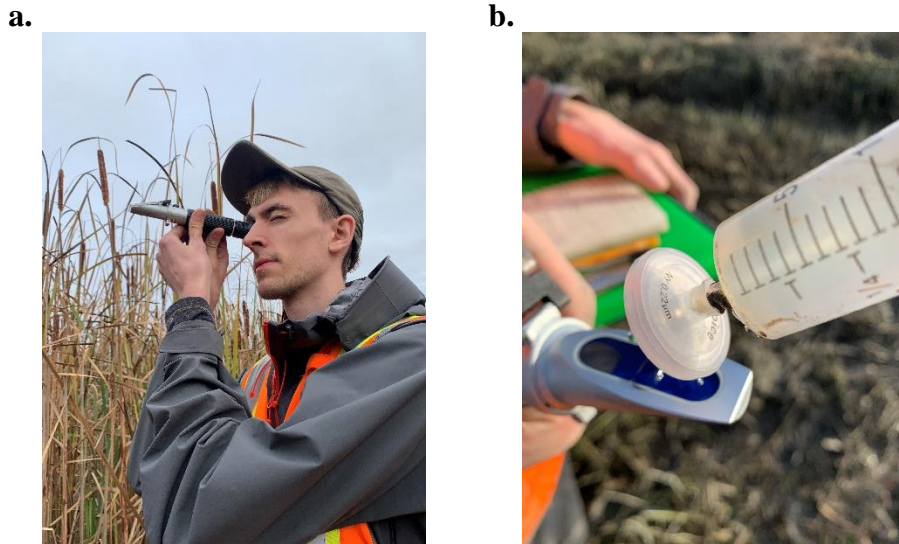
Figure 6. Refractometer reading (a) and refractometer sample preparation (b).
