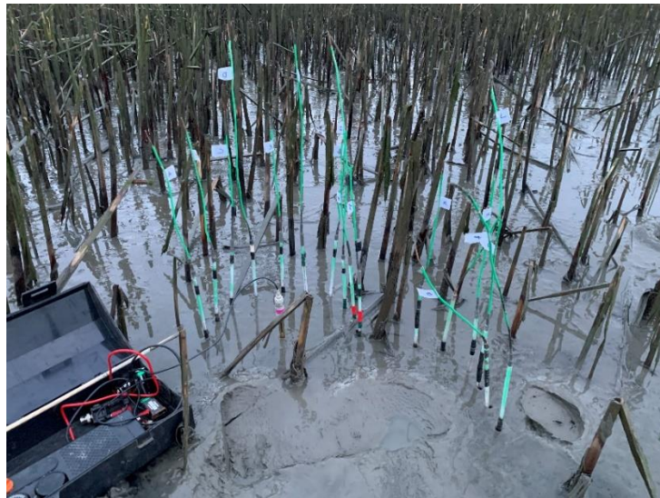
Figure 9. Redox electrodes equilibrating at 2.5cm in the sediment with calomel electrode in the middle. Voltage meter and leads on lower left.
