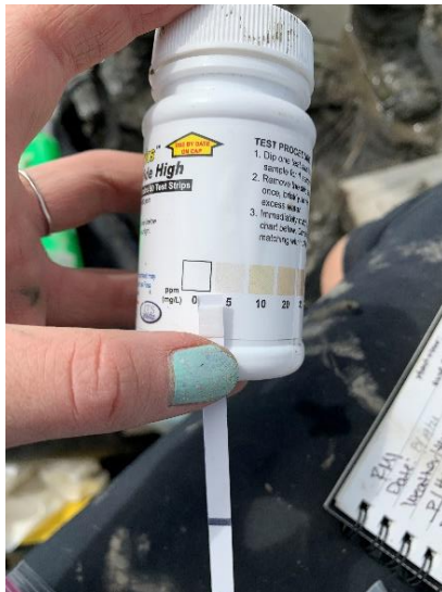
Figure 8. Hydrogen sulfide test strip against color chart.
