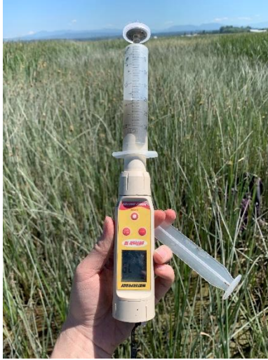
Figure 7. Hand-held meter reading porewater pH.
