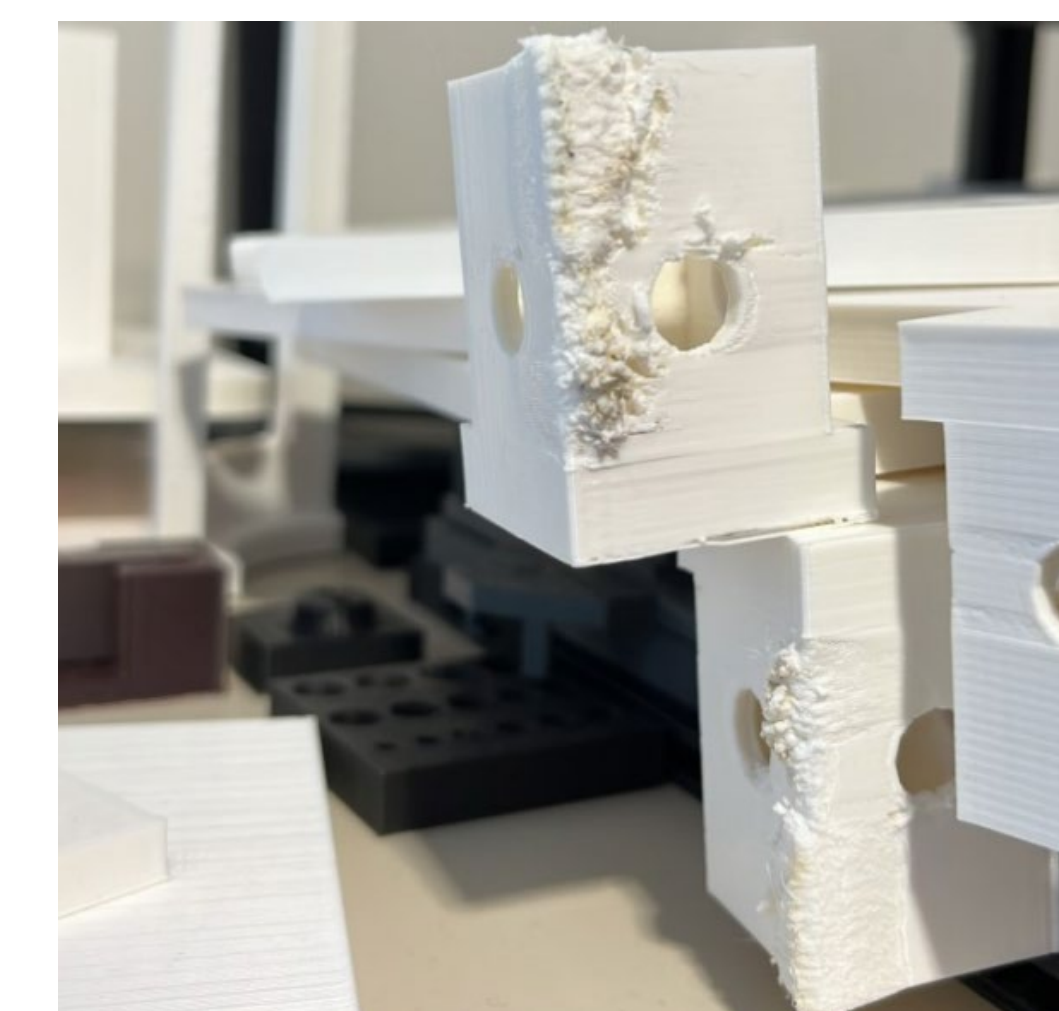
Failed print—operational stress
