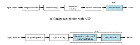
(b) Image recognition with CNN combine dimension reduction, feature extraction, and classification processes
