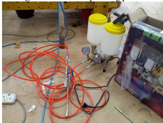
Figure 3. PU injection equipment
