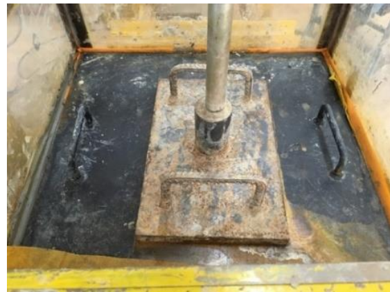
Figure 2. Consolidation process of marine clay
