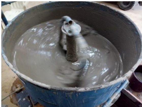
Figure 1. Marine clay mixing process
