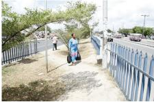
Figure 25. Broken barrier which had been constructed to direct pedestrians to use the overpass bridge along Morogoro Road to avoid accidents and traffic jams. Source: Michuzi blog (Michuzi, 2008).
