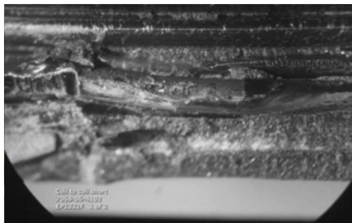
Figure 2.17 An example of the insulation breakdown of motor stator windings [107].
