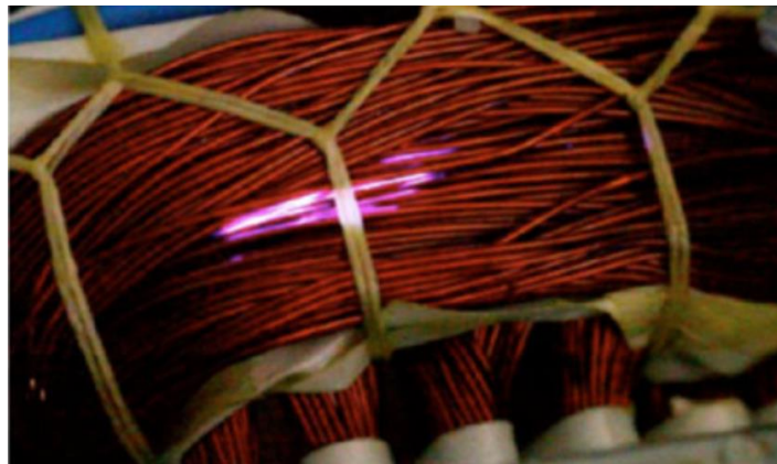
Figure 2.16 PD activity in motor stator windings [106].
