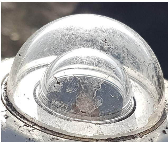
FIGURE 14 Pyranometer dome after artificial soiling on 19 January [Colour figure can be viewed at wileyonlinelibrary.com ]
