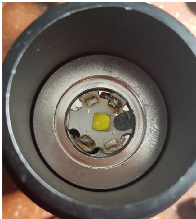
FIGURE 2 LED, connections, and PT100 temperature sensor (covered with thermo-paste) [Colour figure can be viewed at wileyonlinelibrary.com ]
