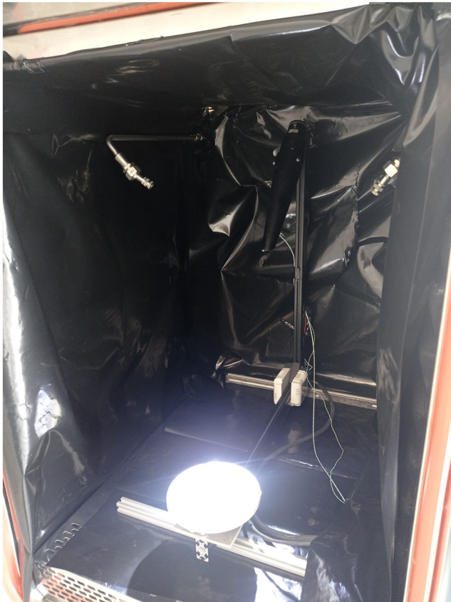
FIGURE 5 Setup for testing the temperature dependence of the lamps in a Vötsch-ATLAS SC340_MH climate chamber [Colour figure can be viewed at wileyonlinelibrary.com ]
