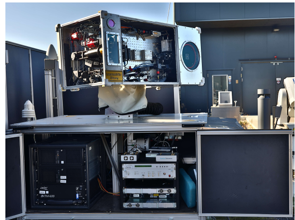
Fig. 4. Open view of the miniSLR ® 3.0. The lids are detached on the front and side to allow a glimpse inside the miniSLR ® . In the top compartment the left side encloses the transmitter, the right side the telescope and in between mainly laser, parts of the receiver and USB electronics are placed. The bottom compartment holds computers and mount controller on the left and electronics for e.g. timing, GPS and internet on the right
