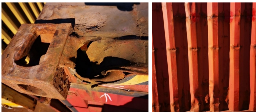
Figure 1. Examples of damaged containers due to external impacts.
