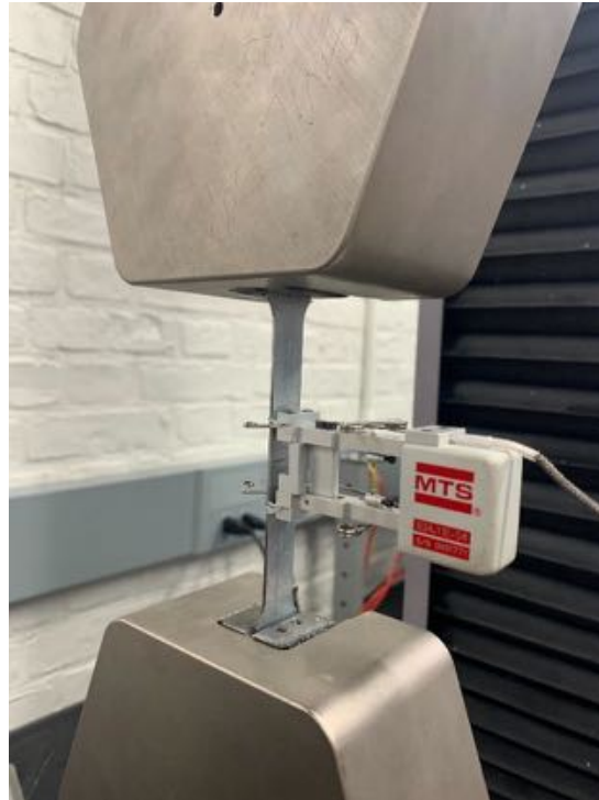
Figure 17. Tensile test of deck coupon
