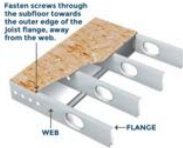
Figure 5. Cold-formed steel joists rendering [6]
