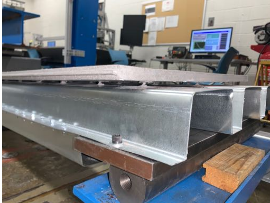
Figure 33. Uplift of structural panel due to shear failure of the panel fasteners
