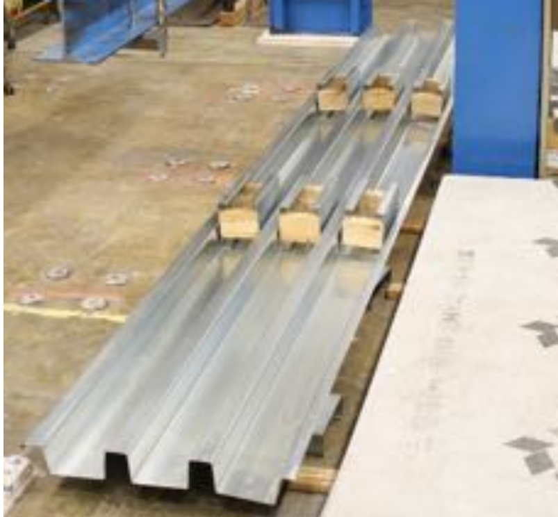
Figure 10. Stiffeners placed inside the specimen during fabrication
