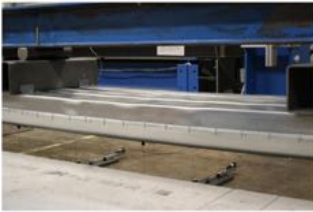
Figure 23. Initial buckling and yielding in the top deck of a bare steel deck specimen
