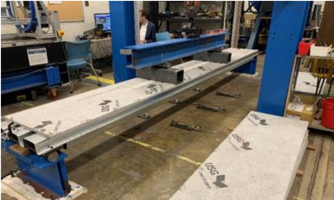
Figure 2. Four-point bending lab setup
