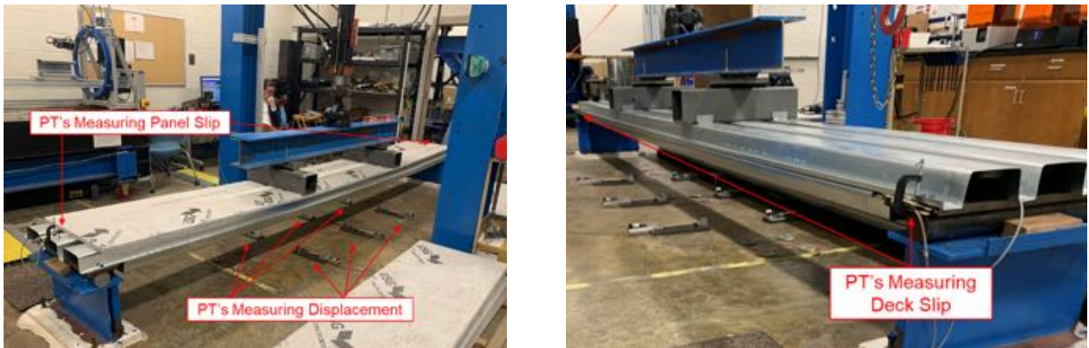
Figure 15. Position transducer locations
