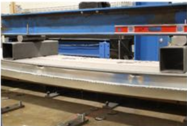
Figure 26. Panel fasteners begin failing in shear as peak load is reached
