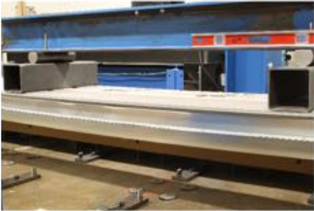
Figure 25. Initial buckling and yielding in the top deck of a specimen with cementitious panel
