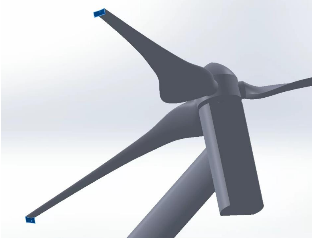
Figure 7-2: GOE 447 blades with downstream-facing winglets
