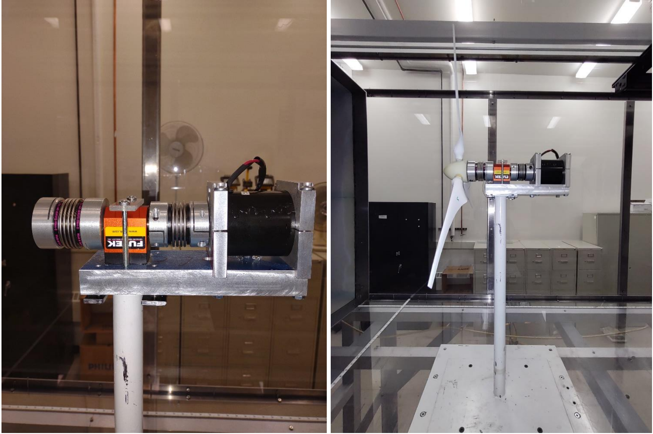
Figure 8-4: (left) the actual built power measurement setup details, (right) side view of the straight blade model.
