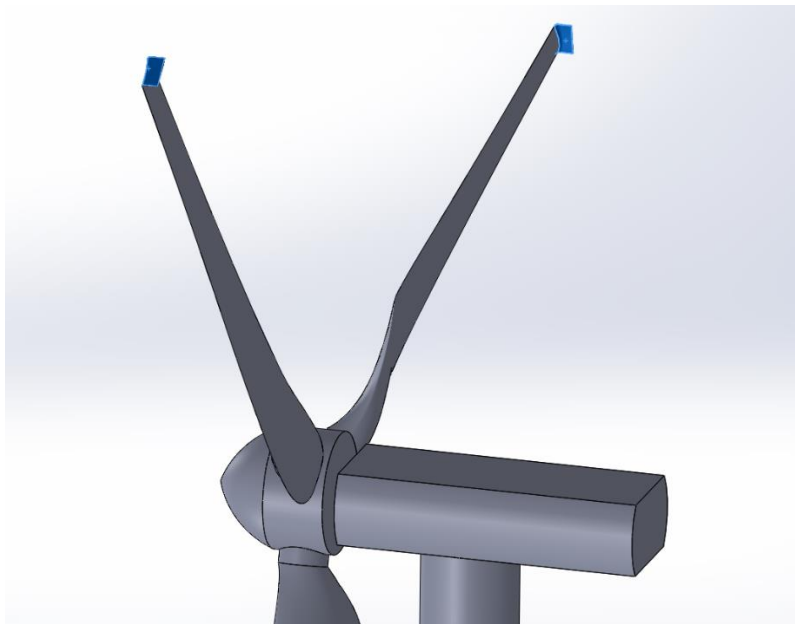
Figure 6-6: GOE 447 blades with suction-side vortex generators
