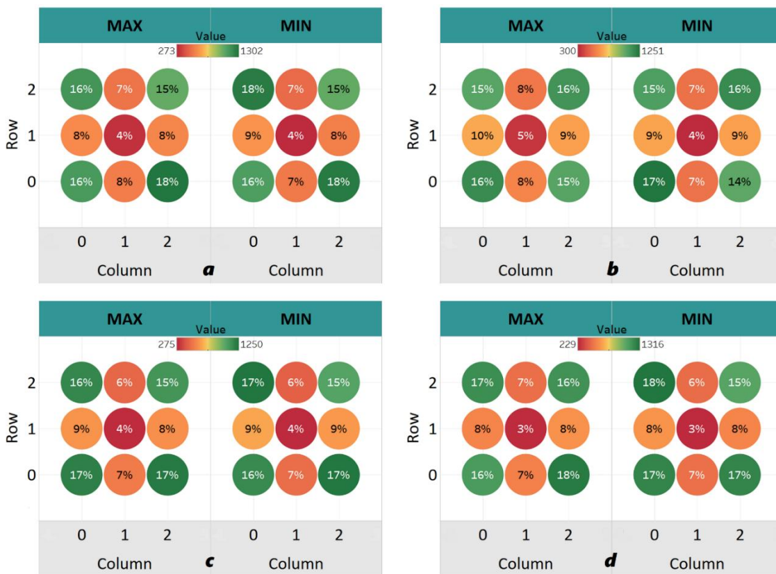
Figure 6.6. Position of the min and max values in 3x3 pixel sub matrices subject to NaOH sonicated at amplitudes (a) 30%, (b) 50%, (c) 70% and (d) 90% of the maximum power
