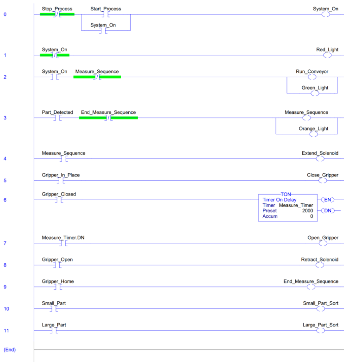
Figure 9: PLC ladder logic Program for example application
