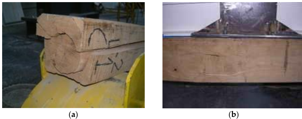
Figure 6. Failure modes: (a) unreinforced timber beam; (b) reinforced beam.
