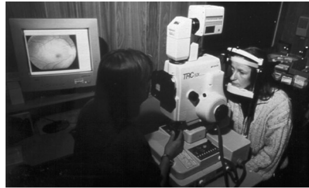
FIGURE 2 Topcon retinal camera with IMAGENet system
