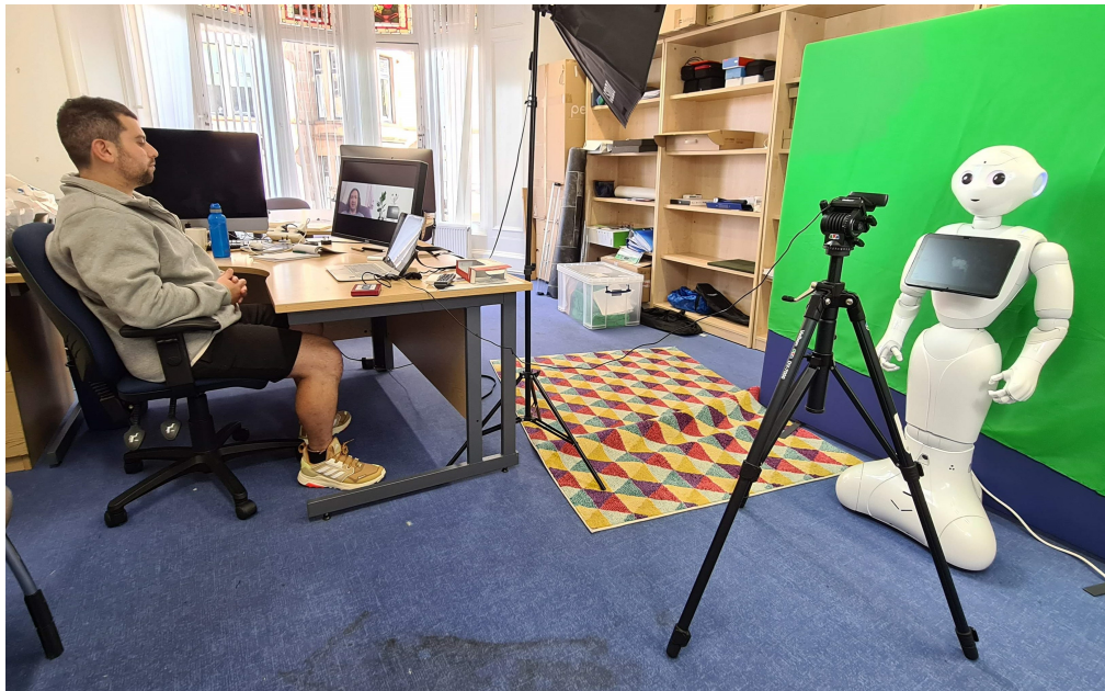
Figure 2: The lab settings, including the robot Pepper (SoftBank Robotics) in front of a web camera, while the experimenter in the back is controlling the robot using the Wizard of Oz technique.
