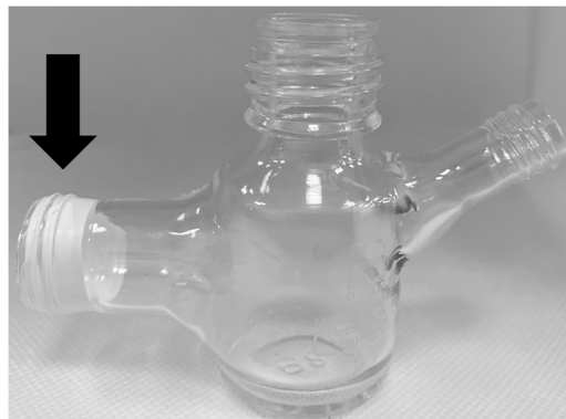
Figure 2. Teflon tape used at the threading of the compartment joint to prevent leakage
