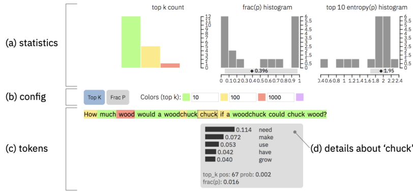
Fig. 29: An example of the GLTR interface. The system displays global statistics about the input, including information as to the distribution of common and uncommon terms. The system also provides intuitions as to how likely a given term is relative to the most probable terms. Retrieved from [220].
