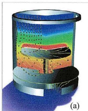
Viscous drag forces uniformly deposit compound semiconductor materials on wafers
