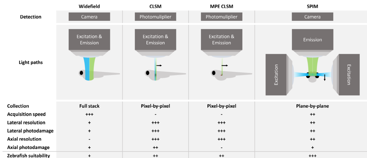
Fig. 1. Fluorescence microscopy in zebrafish imaging. Widefield fluorescence microscopy images the whole field-of-view without filtering out-of-focus light, resulting in relatively high acquisition speeds and low photodamage at the cost of lateral and axial resolution. CLSM uses a pinhole for optical sectioning, resulting in relatively high resolution at the cost of increased photo-damage and decreased acquisition speeds, due to the need of pixel-by-pixel scanning of a powerful laser. Axial photodamage can be reduced in MPE where excitation only occurs in the focal plane. In SPIM, the detection light path is perpendicular to the illumination light path allowing increased acquisition speeds and decreased photodamage.
