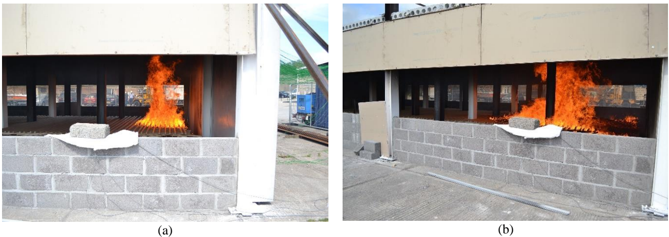
Figure 5: Fire development and temperatures recorded at different intervals along the length of the test compartment: (a) early fire development; (b) fully developed fire in the middle of test compartment
