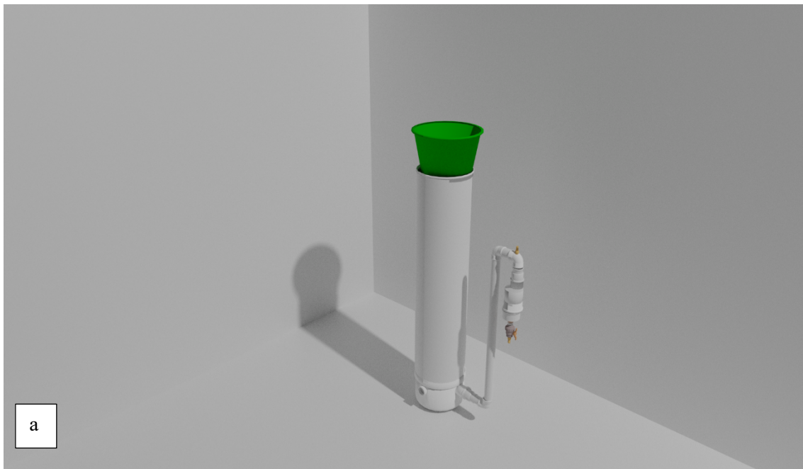
Figure S2 – Intermittent (a) and continuous (b) HSSF design. Continuous HSSF requires bigger infrastructure and occupies more area compared to intermittent.
