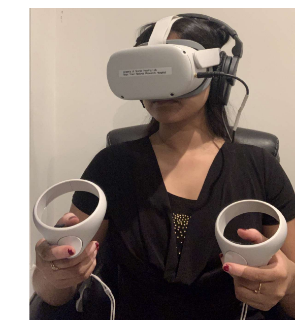
Figure 5: A standalone VR headset (Oculus Quest 2) along with calibrated circumaural headphones (Sennheiser HD 280) were used to deliver auditory and visual stimuli.
