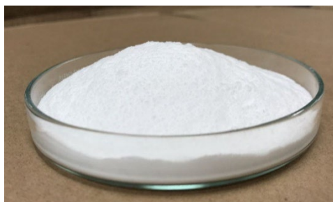
Figure 3.1. Appearance of “dry water” synthesized from hydrophobic silica “H18” and deionized water.
