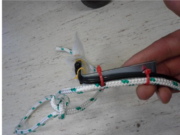
Fig. 2. Leaf wetness sensor connected to angled bracket and rope.
