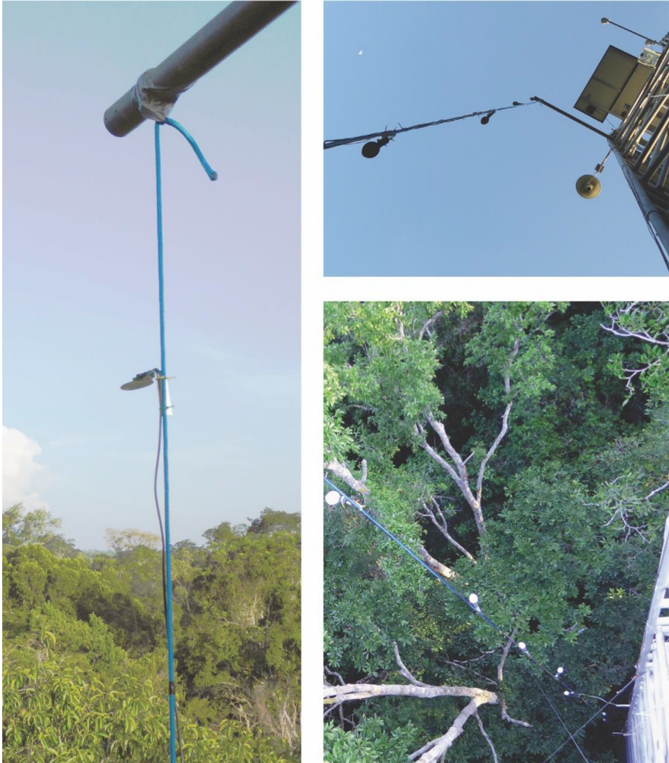
Fig. 1. Picture of a leaf wetness sensor 'rig'. The panel on the left shows the attachment of the supporting rope to the scaffold pole which is mounted on the meteorological tower. The panel on the right shows a view looking upwards including the tower and the rig.
