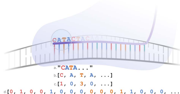
Figure 2. Four different ways to encode the sgRNA nucleotide sequence. Demonstrated are the four encircled nucleotides (CATA): (A) as a string—this will not be compatible with many ML algorithms; (B) as a list of characters—here, each nucleotide has its own 'feature'. However, many ML algorithms require features to be represented as numbers; (C) as a list of numbers—here, each nucleotide has been arbitrarily assigned a value from 0 to 3. However, algorithms that accept 'continuous' features will consider T (3) to be more different from A (0), than T is from G (2) because of the larger difference in the arbitrarily assigned values; (D) one-hot encoded—here, each nucleotide is represented as four list elements. One (and only one) of these elements is 'hot' (i.e. 1) depending on the nucleotide. In this example, the first element being hot, i.e. [1, 0, 0, 0], represents an A. In this representation, all nucleotides are represented as being equally different.
