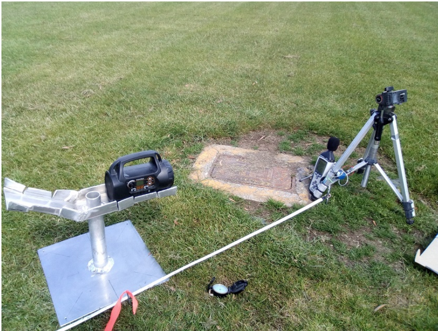
Figure 6.3: Testing the detection range of an ABAR. On the the leftmost leg of the big tripod we secured a SOROKA 15E with external battery and microphone. Beside this, the smaller tripod holds the SPL meter in place whilst a tape measure runs between a movable aluminium platform (the same as in chapter 3) onto which lays a FoxPro NX4 speaker. We used a compass to have the tape measure always in the same direction for reproducibility in case we needed to repeat the tests. The testing track included two NIBK vocalisations (one per sex). In the actual test we broadcast these vocalisations at natural amplitude (Castro et al., 2019) at increasing distances along the tape measure to ascertain the distance at which a NIBK vocalisation would not be detected by the ABAR.
