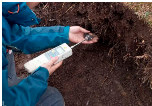
Figure 4. Measuring the maximum pullout force of individual roots using a tension meter.
