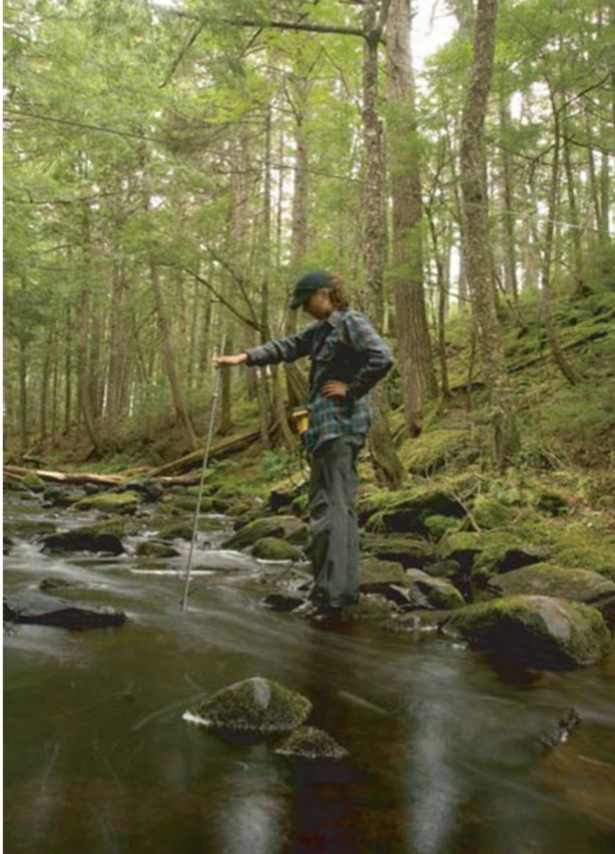
Figure 9. Liz Johnson performing velocity measurements using a Marsh-McBirney flow meter on Baker Brook in the Narraguagus River Watershed, ME (from Johnson, 2009).
