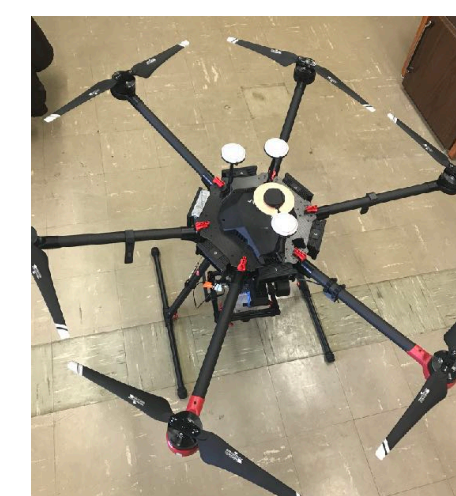
Figure 7: DJI Matrice 600 Drone that will be used to collect hyperspectral data in the future
