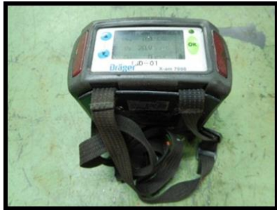
Gambar 7. Portable Gas Detector DRAGER type X-AM 7000
