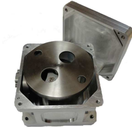
Figure 15. Reaction wheel unit from SSDC lab at Ryerson University. [2]
