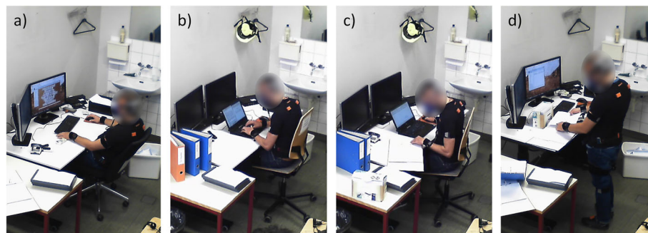
Fig. 1 Investigated workplaces and tasks. Participant using the conventional chair (a), the activity-promoting chair (b and c), and the standing desk (d) to complete the four tasks Mouse (a), Keyboard (b), Deskwork (c), and Sorting (d). Picture b and c show a participant using the laptop
