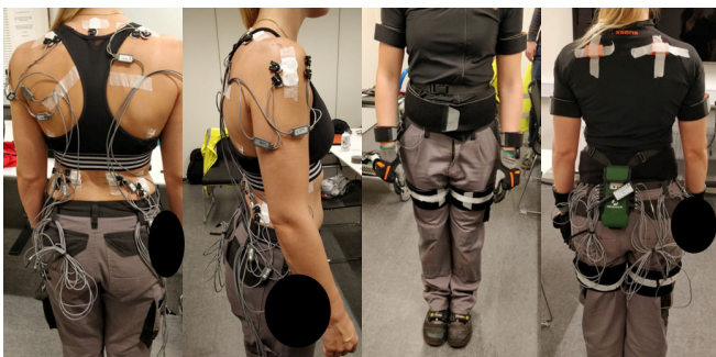
Fig 1. Experimental setup with sEMG and IMU sensors.
