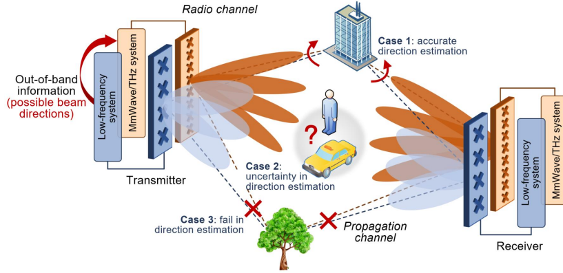
Fig. 1. The schematic of using out-of-band spatial channel information for fast mmWave/THz beam search.
