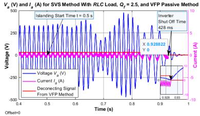
Fig. 16. Inverter response under islanding with SVS method and  $K_{SVS} = 1$  A/V: PCC voltage, PCC current, and fault disconnecting signal.
