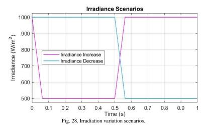
Considering the solar irradiation variation as depicted in Fig. 28, the PCC grid voltage and current of the studied active islanding methods for increasing and decreasing irradiance will be represented in Fig. 29. Fig. 30 illustrates the active and reactive power for increasing and decreasing in irradiance, while Fig. 31 shows the frequency and ROCOF for increasing and decreasing irradiance. From the obtained results, it can be concluded that studied IDMs
