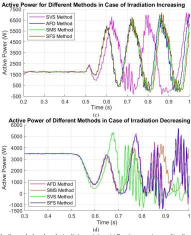
Fig. 30. Studied active islanding methods under solar irradiation variations. (a) Reactive power in case of irradiance increases. (b) Reactive power in case of irradiance decreases. (c) Active power for irradiance increasing. (d) Active power for irradiance decreases.
