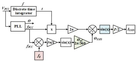
Fig. 6. SMS method block diagram.
