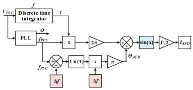
Fig. 2. AFD method block diagram.
