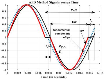
Fig. 1. Simulated waveform used by the AFD method [30], [85].
