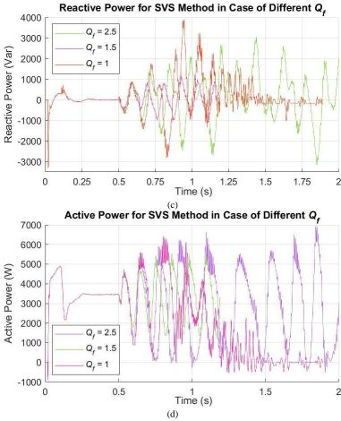
(d) Fig. 22. Obtained results for SVS method at different  $Q_f$ . (a) RMS grid current. (b) RMS grid voltage. (c) Reactive Power. (d) Active power.
