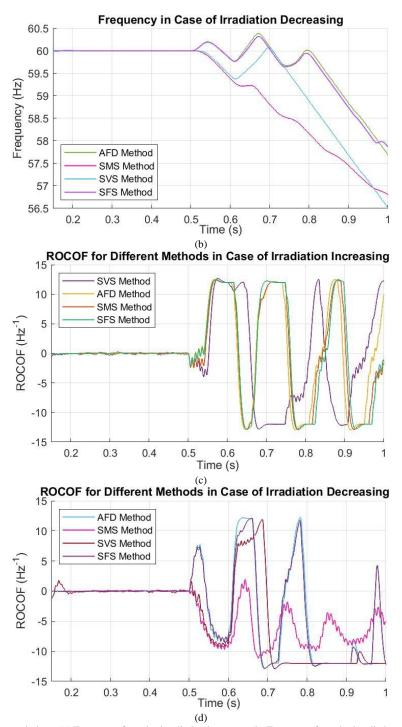
Fig. 31. Solar irradiance variations. (a) Frequency for solar irradiation increases. (b) Frequency for solar irradiation decreases. (c) ROCOF for solar irradiation decreasing.
