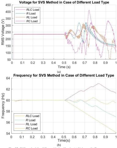
Fig. 27. SVS method for different kinds of loads. (a) Voltage. (b) Frequency.
