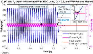
Fig. 14. PV inverter response under islanding with SFS method and  $K_{SFS} = 0$  Hz<sup>-1</sup>: PCC voltage, PCC current, and disconnecting signal.
