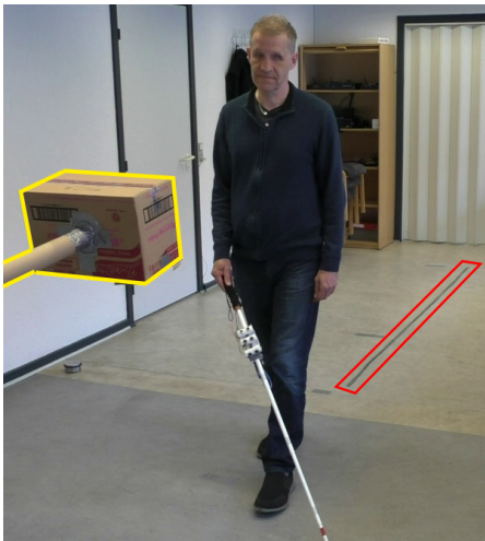
Figure 2: Picture of the setup: red - trail created from folded tape. yellow - the boxes used as obstacles
