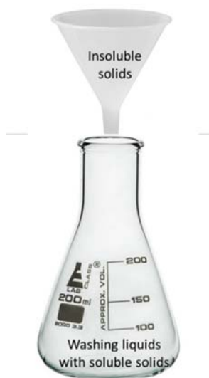
Figure 3-17 Gravitational filtration set-up for the washing of the okara. A filter (Whatman #1) was used with the funnel to collect insoluble solids, and the washing liquids was later dried to collect the soluble solids.
