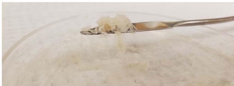
Figure 3-29 Appearance of the dried solids present in the liquid layer generated during the ultracentrifugation of citric acid treated okara. Clear sticky flakes.
