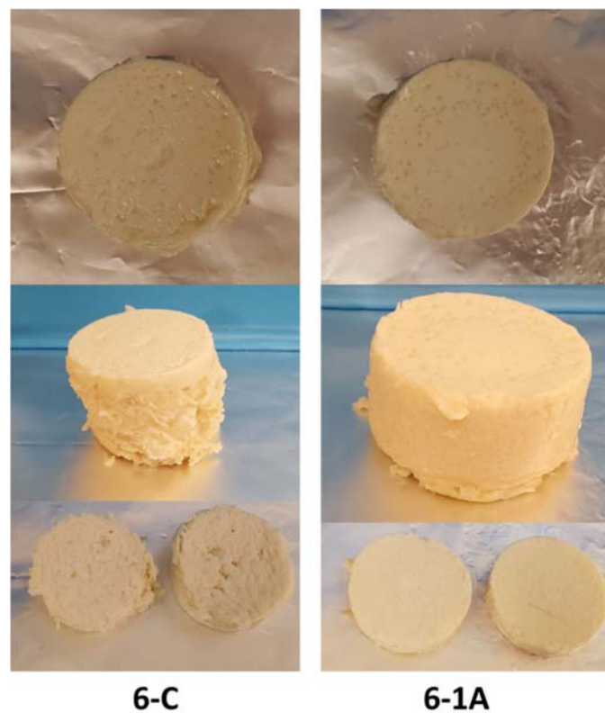
Figure 3-24 Physical appearance of control sample (6-C) (100% wet, untreated okara) and sample 6-1A (heat-treated okara). Sample 6-1A was significantly more homogeneous and had higher gel strength.
