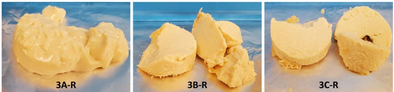
Figure 3-6 Physical appearance of replicate samples 3A-R, 3B-R, and 3C-R from left to right. Samples were cooled at room temperature. Samples were completely set.
