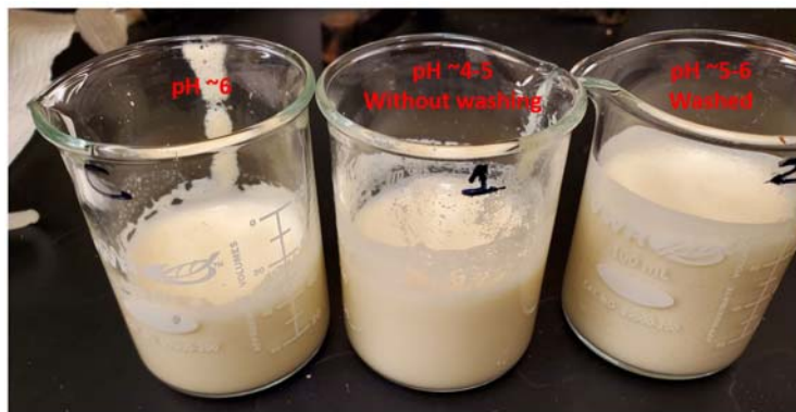
Figure 3-9 pH of control sample, 4-C (left, 100% wet okara added to soymilk), and samples 4A (middle, labelled as 1) and 4B (right, labelled as 2), prior to heat treatment. Heavy foam was noted on top of sample 4B, which could have attributed to the gel's large pore size.
