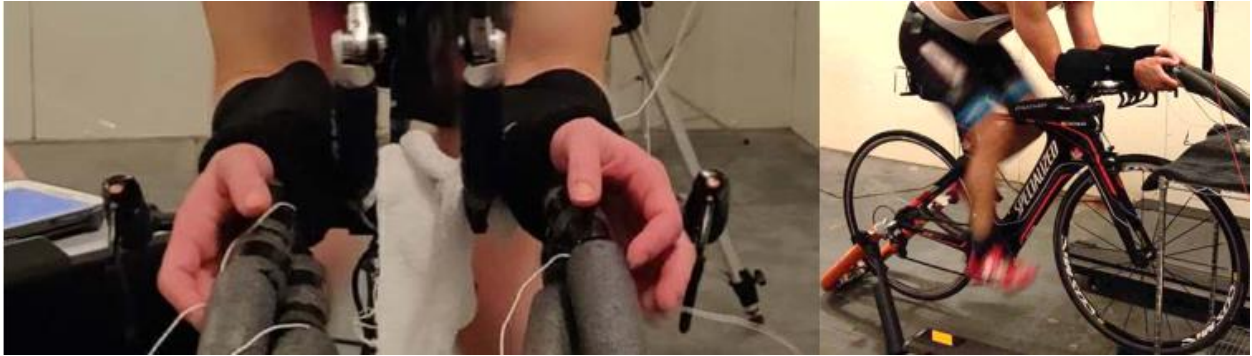
Figure 3.3: Arrangement of the cooling system when affixed to participants arms.
