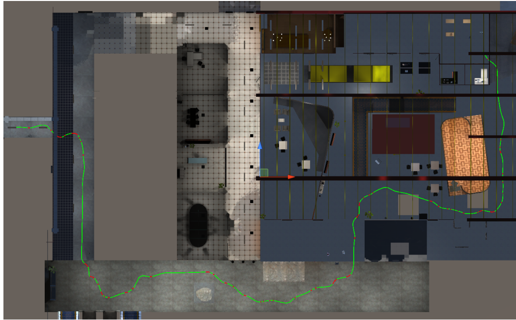
Figure 8. An example path taken by the robot. The green line shows the robots autonomous movement, and the red line shows the robots movement when it is controlled by the user.
