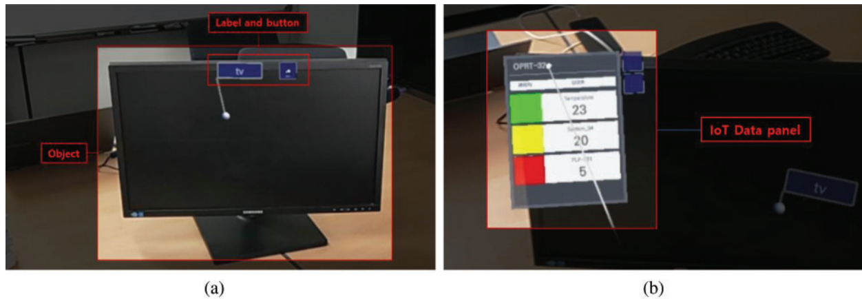
Figure 11: Marker-less M2MR System (a) Faster R-CNN-based OT and UI (b) Demonstration of the IoT panel
